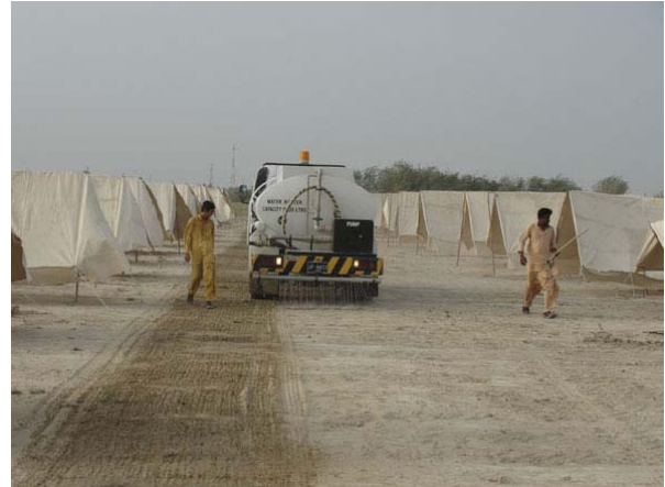
Water bowser sprinkling water to settle the dust
